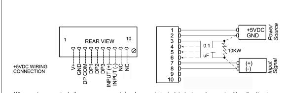
When systems require both power source and signal source to be isolated, please be sure to either directly wire or connect through a 10KW resistor, 0.1uF capacitor, pins two (2) and (8). By doing this, errors caused by ground loops will be reduced. The pins that are not being used need to be left open.
