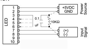
When systems require both power source and signal source to be isolated, please be sure to either directly wire or connect through a  $10 \mathrm{K}\Omega$  resistor, 0.1uF capacitor, pins two (2) and (8). By doing this errors caused by ground loops will be reduced. The pins that are not being used need to be left open.
